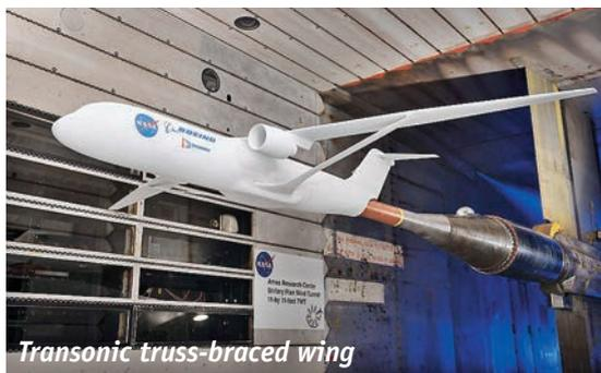
Transonic truss-braced wing
